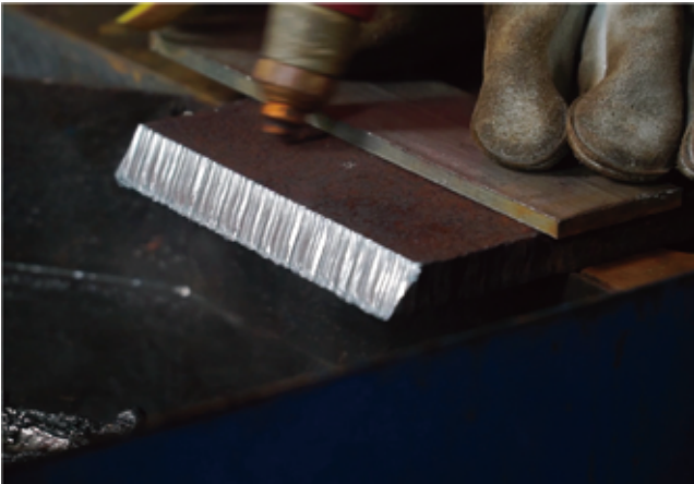
*16mm M.S. 60° bevel cutting by PROCUT-75MAX
